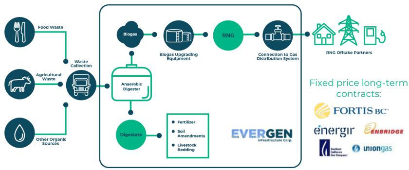
Feedstock is supplied to the anaerobic digester which contains bacteria that breaks down organic matter in the absence of oxygen
